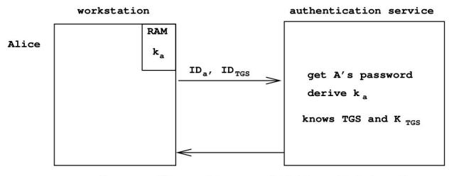
$\{k_{a,\,TGS}\ ,\ ID_{\,TGS}\ ,\ time_{\,kdc}\ ,\ lifetime,\ ticket_{\,TGS}\}k_{a}$
