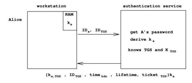
ticket  $_{TGS} = \{k_{A, TGS}, ID_A, time_{KCD}, lifetime, ID_{TGS}, addr_A\}k_{TGS}$
